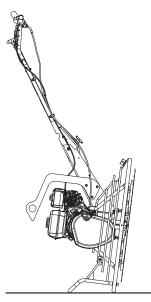
*NOTICE* Do not tilt the machine in any other direction. Incorrect tilting or leaning can cause problems with engine oil pouring out through the valve into the carburettor.
