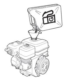
4. Never overfill the tank. Due to the movement of the fuel within the tank, it is possible to have fuel at a higher level than the tank cap, which can lead to a spillage of fuel if the tank cap is opened. This can be avoided by only opening the tank cap when the machine is on level ground and the tank cap is at the fuel tank's highest point.
