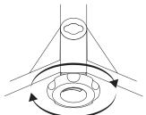
To decrease the blade angle, turn the twist pitch knob counterclockwise.
